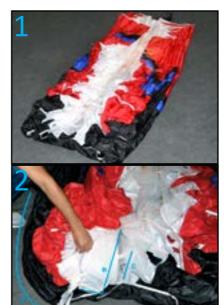
Step 1. Open the canopy completely on the ground and fold him in form of a accordion, though you avoid dragging him over the ground.
