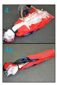
Step 4. Organize the canopy in form of o accordion of both sides and then put one side up the other. Now all battens should be positioned lateral.
