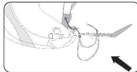
The incorrect installation of the foot stirrup may prevent the reserve parachute opening. Make sure that does not happen.
