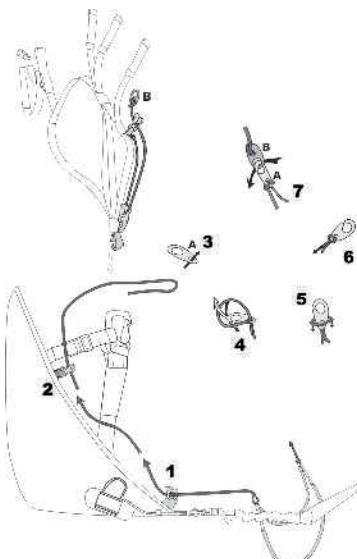
The necessary pulleys to adjust the speed system are in the harness itself. The cables must be initially passed through the pulleys in front of the seat.
