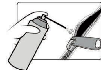
In most cases, you will be able to repair the zipper yourself. In case the slider is not able to close the zipper, bring it to the starting point and with some pliers tighten the slider on both sides.
