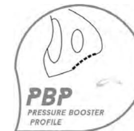
A new profile design to increase the wing pressure, resulting in form stability. More performance along the whole speed range is the result.
