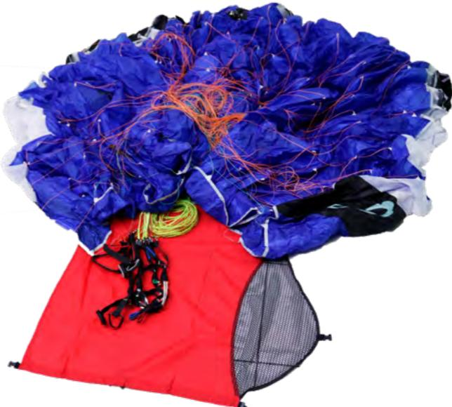
Step 1: Open the origami sack and pull the partially in. The outside will look like a cabbage. This way you're avoiding that the glider drags over the ground during folding.
