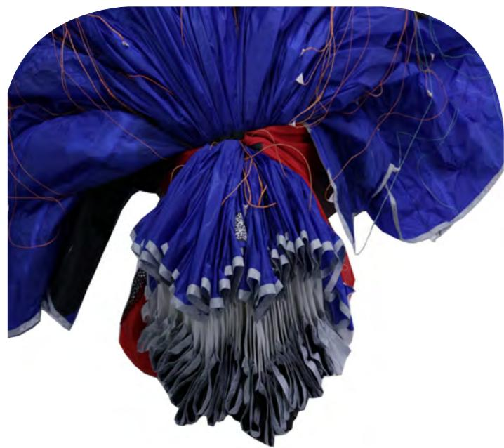
Step 4: Fold the wing like an accordion from both sides and close the origami sack. Watch out for the lines and fabric closing the zipper.
