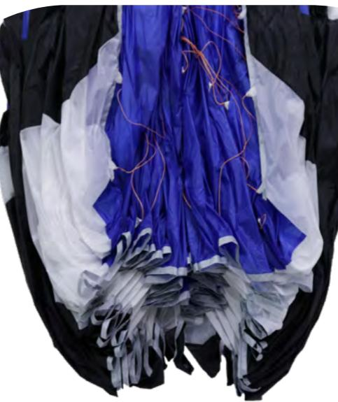
Step 1: Bundle up your glider in form of a cabbage. This way you're avoiding that the glider drags over the ground during folding.
