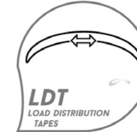
LDT are Load Distribution Tapes between the suspension points for a weight distribution along the whole wing during flight, resulting in better performance and stability.
