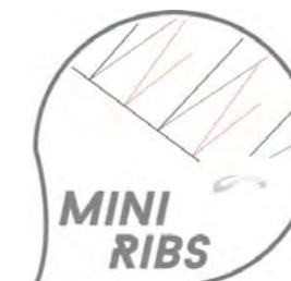
Profiles between the cells of the trailing edge, resulting in better performance and handling.
