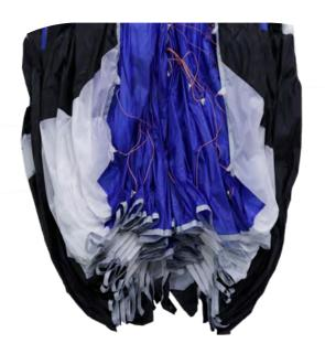
Step 3: Now do it in the same way with the leading edge profiles. Put the reinforcements of top and bottom in the right way, don't close the cell openings and push out the fabric.
