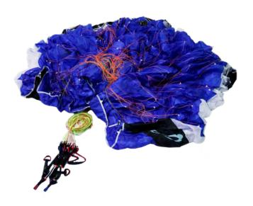
Step 1: Bundle up your glider in form of a cabbage. This way you're avoiding that the glider drags over the ground during folding.
