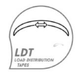
LDT are Load Distribution Tapes between the suspension points for a weight distribution along the whole wing during flight, resuLT 1ing in better performance and stability.
