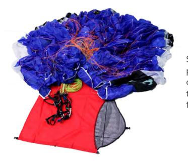
Step 1: Open the folding bag and pull the partially in. The outside will look like a cabbage. This way you're avoiding that the glider drags over the ground during folding.
