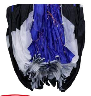
Step 3: Now do it in the same way with the leading edge profiles. Put the reinforcements of top and bottom in the right way, don't close the cell openings and push out the fabric.
