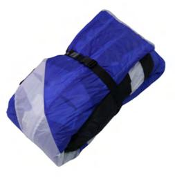
Step 5: Fold the sack as shown in the photo. This method is very gentle to the more stiffer parts of the mini wing.
