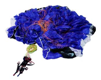
Step 1: Bundle up your mini wing in form of a cabbage. This way you're avoiding that the mini wing drags over the ground during folding.
