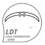
LDT are Load Distribution Tapes between the suspension points for a weight distribution along the whole wing during flight, resulting in better performance and stability.
