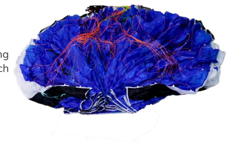
Step 3: Now do it in the same way with the leading edge profiles. Put the reinforcements of top and bottom in the right way, don't close the cell openings and push out the fabric.
