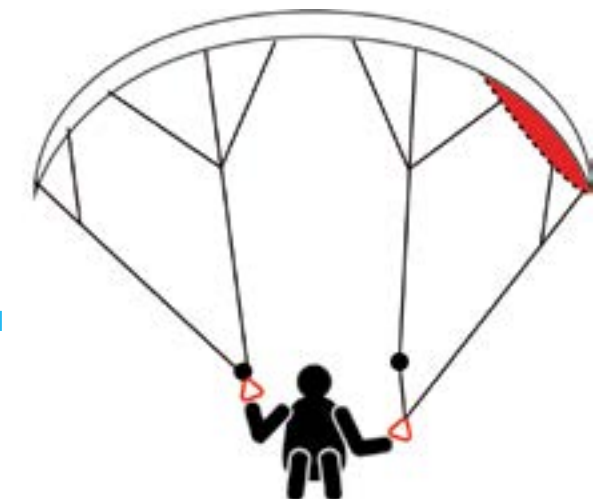
Closed turn – Pull one of the commands downwards close to your body.
