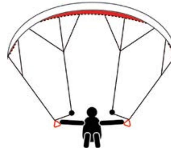
Intense speed reduction Recommended for landings and starts. Pull the two commands horizontally downwards to the side.
