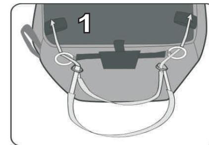
The lines of the speed system need to be passed through the rings to avoid problems in case of rescue deployment.
