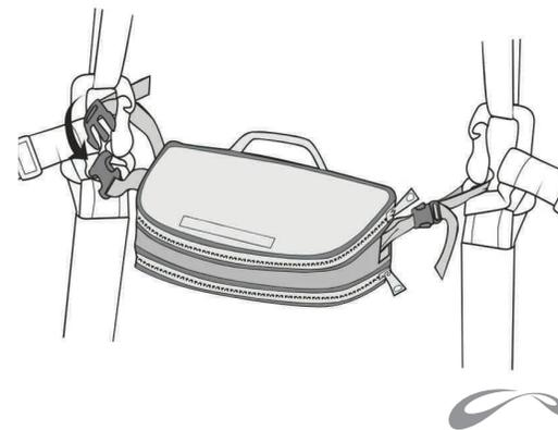
**SOL Harness** line allows for the attachment of a special reservoir ( container ), where the pilot may carry his / her electronic instruments during flight.
