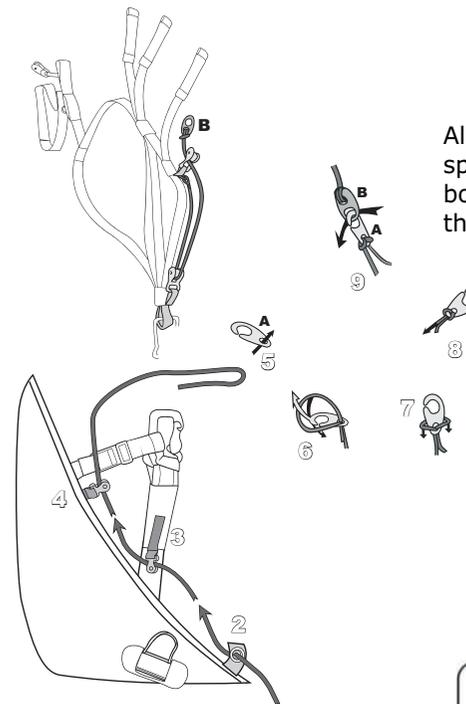
All necessary buckles to adjust the speed system are found on the harness' body. The cables must be fed initially through the pulleys in front of the seat.
