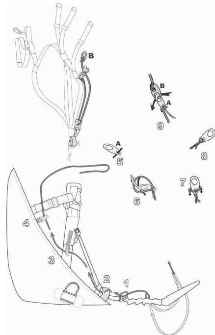
The lines of the speed system need to be passed through the rings to avoid problems in case of rescue deployment.
