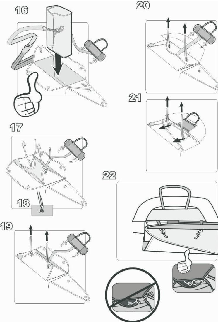
**SOL Harness** features a reserve parachute installation system with easy access at the moment of grab and throw, by possessing an activator which has a shorter connection.
