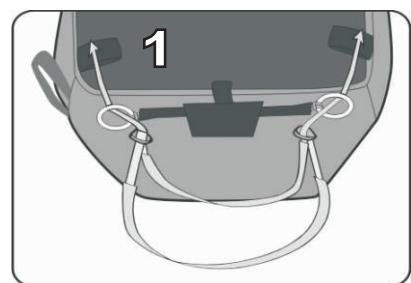
All necessary buckles to adjust the speed system are found on the harness' body. The cables must be fed initially through the pulleys in front of the seat.
