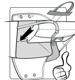
The reserve parachute compartment on your harness was designed for most of the parachutes in the market. In any case, you must install, simulate and perform all testing, so that you will not have any surprises in case you need to activate it. Any questions concerning its operation must be dealt with during the installation and setting of the harness before the first flight.
