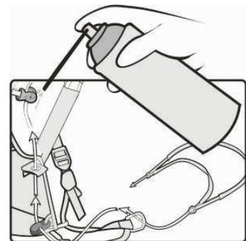
It is very important to maintain all pulleys, Carabiners, Auto Buckles well lubricated, as this will keep from stressing the speed system lines and axel.
