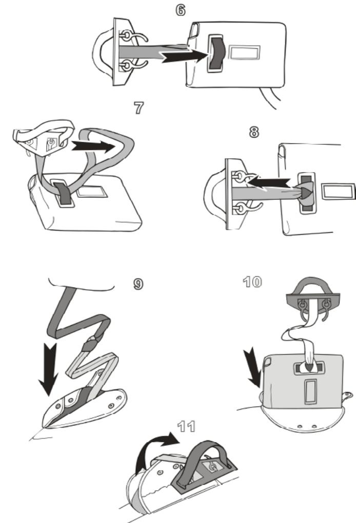
Some layers of Cordura® cover the recipient entry which is destined to the reserve (Figure9), protecting the parachute against dust and humidity.
